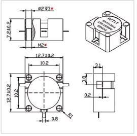
RF Solution offer a wide selection of Drop in Circulator for global customers. WH1313M is a Drop in Circulator in Frequency Range of 800~7000 MHz. It is made of high quality materials under a high standard, the Bandwidth Max of this product is 10%, Insertion Loss Max is 0.30~0.50 dB and Isolation Min is 18.0~23.0 dB. The component has a good working performance and stability, it is ideal for handling a Power of 50 W.
