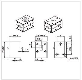
RF Solution offer a wide selection of Broadband Circulator for global customers. WH1319C is a Broadband Circulator in Frequency Range of 6.0~12.0 GHz. It is made of high quality materials under a high standard, the Bandwidth Max of this product is 100%, Insertion Loss Max is 0.50~0.60 dB and Isolation Min is 16.0~18.0 dB. The component has a good working performance and stability, it is ideal for handling a Power of 30 W.
