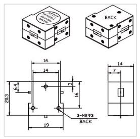
RF Solution offer a wide selection of Drop in Circulator for global customers. WH1620B is a Drop in Circulator in Frequency Range of  $6.0 \sim 18.0$  GHz. It is made of high quality materials under a high standard, the Bandwidth Max of this product is 100%, Insertion Loss Max is  $0.50 \sim 1.50$  dB and Isolation Min is  $10.0 \sim 20.0$  dB. The component has a good working performance and stability, it is ideal for handling a Power of 30 W.
