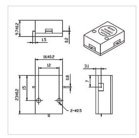
RF Solution offer a wide selection of Drop in Circulator for global customers. WH1623D is a Drop in Circulator in Frequency Range of 5.0~7.0 GHz. It is made of high quality materials under a high standard, the Bandwidth Max of this product is 20%, Insertion Loss Max is 0.40~0.60 dB and Isolation Min is 18.0~23.0 dB. The component has a good working performance and stability, it is ideal for handling a Power of 50 W.
