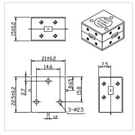
RF Solution offer a wide selection of Drop in Circulator for global customers. WH2123B is a Drop in Circulator in Frequency Range of 4.0~8.0 GHz. It is made of high quality materials under a high standard, the Bandwidth Max of this product is 100%, Insertion Loss Max is 0.40~0.60 dB and Isolation Min is 18.0~19.0 dB. The component has a good working performance and stability, it is ideal for handling a Power of 100 W.
