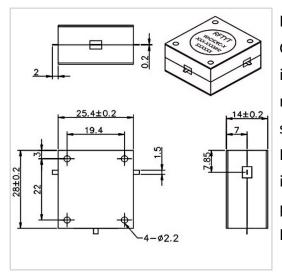
RF Solution offer a wide selection of Drop in Circulator for global customers. WH2528C is a Drop in Circulator in Frequency Range of 3.0~6.0 GHz. It is made of high quality materials under a high standard, the Bandwidth Max of this product is 100%, Insertion Loss Max is 0.40~0.50 dB and Isolation Min is 18.0~20.0 dB. The component has a good working performance and stability, it is ideal for handling a Power of 150 W.
