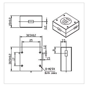
RF Solution offer a wide selection of Drop in Circulator for global customers. WH3030B is a Drop in Circulator in Frequency Range of 2.0~6.0 GHz. It is made of high quality materials under a high standard, the Bandwidth Max of this product is 100%, Insertion Loss Max is 0.85~1.70 dB and Isolation Min is 12.0 dB. The component has a good working performance and stability, it is ideal for handling a Power of 50 W.
