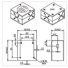
RF Solution offer a wide selection of Drop in Circulator for global customers. WH3234A is a Drop in Circulator in Frequency Range of 2.0~4.0 GHz. It is made of high quality materials under a high standard, the Bandwidth Max of this product is 100%, Insertion Loss Max is 0.40~0.50 dB and Isolation Min is 18.0~20.0 dB. The component has a good working performance and stability, it is ideal for handling a Power of 150 W.
