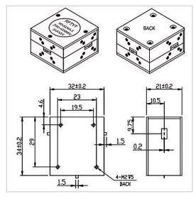
RF Solution offer a wide selection of Drop in Circulator for global customers. WH3234B is a Drop in Circulator in Frequency Range of 2.0~4.20 GHz. It is made of high quality materials under a high standard, the Bandwidth Max of this product is 100%, Insertion Loss Max is 0.50~0.60 dB and Isolation Min is 18.0~19.0 dB. The component has a good working performance and stability, it is ideal for handling a Power of 150 W.
