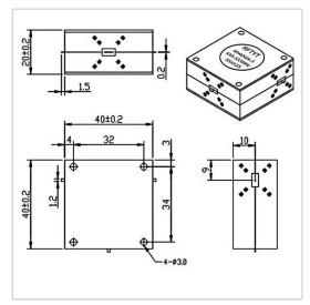
RF Solution offer a wide selection of Drop in Circulator for global customers. WH4040A is a Drop in Circulator in Frequency Range of 1.50~3.5 GHz. It is made of high quality materials under a high standard, the Bandwidth Max of this product is 100%, Insertion Loss Max is 0.60~0.70 dB and Isolation Min is 17.0~18.0 dB. The component has a good working performance and stability, it is ideal for handling a Power of 100 W.
