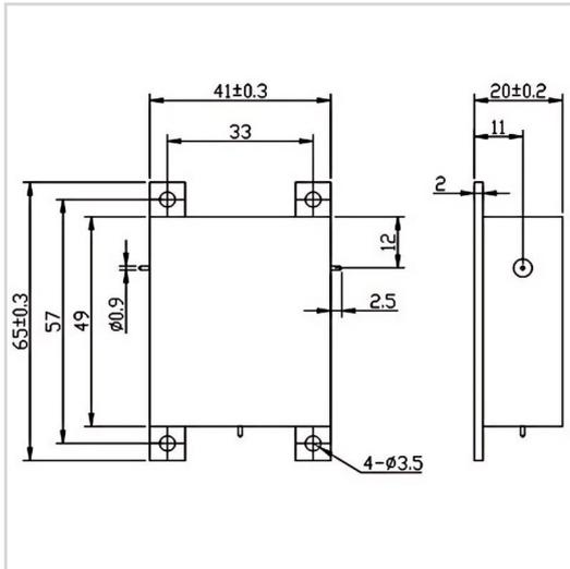
RF Solution offer a wide selection of Drop in Circulator for global customers. WH4149A is a Drop in Circulator in Frequency Range of 300~1000 MHz. It is made of high quality materials under a high standard, the Bandwidth Max of this product is 20%, Insertion Loss Max is 0.70~1.20 dB and Isolation Min is 16.0~20.0 dB. The component has a good working performance and stability, it is ideal for handling a Power of 100 W.
