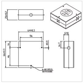
RF Solution offer a wide selection of Drop in Circulator for global customers. WH6466K is a Drop in Circulator in Frequency Range of 950~2000 MHz. It is made of high quality materials under a high standard, the Bandwidth Max of this product is 10%, Insertion Loss Max is 0.65~0.70 dB and Isolation Min is 16.0~17.0 dB. The component has a good working performance and stability, it is ideal for handling a Power of 150 W.
