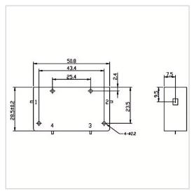
RF Solution offer a wide selection of Dual Junction Circulator for global customers. WHH5028C is a Dual Junction Circulator in Frequency Range of  $3.0\sim6.0$  GHz. It is made of high quality materials under a high standard, the Bandwidth Max of this product is 100%, Insertion Loss Max is  $0.80\sim1.00$  dB and Isolation Min is  $36.0\sim40.0$  dB. The component has a good working performance and stability, it is ideal for handling a Forward Power of  $100\ W$ .
