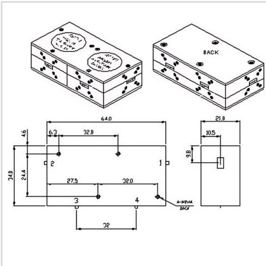
RF Solution offer a wide selection of Dual Junction Circulator for global customers. WHH6434A is a Dual Junction Circulator in Frequency Range of 2.0~4.0 GHz. It is made of high quality materials under a high standard, the Bandwidth Max of this product is 100%, Insertion Loss Max is 1.00~1.20 dB and Isolation Min is 36.0~38.0 dB. The component has a good working performance and stability, it is ideal for handling a Forward Power of 100 W.
