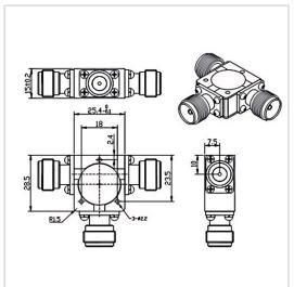
RF Solution offer a wide selection of Coaxial Circulator for global customers. TH2528XN is a Coaxial Circulator in Frequency Range of 700~5000 MHz. It is made of high quality materials under a high standard, the Bandwidth Max of this product is 25%, Insertion Loss Max is 0.30~0.60 dB and Isolation Min is 16.0~25.0 dB. The component has a good working performance and stability, it is ideal for handling a Forward Power of 100 W.
